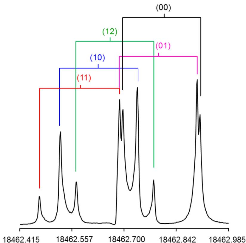
**Figure 4:** A spectrum of the  $8_{35} \leftarrow 7_{34}$  transition of 34DMFB recorded at high resolution which splits into the (00), (01), (10), (11), and (12) torsional species. The frequencies are given in MHz. The Doppler doublets are marked by brackets.
