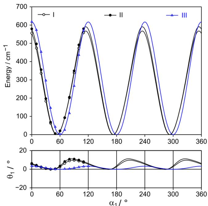
**Figure 2:** Upper trace: Potential energy curves of three conformer of methyl n-propyl sulfide obtained by rotating the thiomethyl group while all other geometry parameters were optimized at the MP2/6-311++G(d,p) level of theory. The energies are given relative to the lowest energy
