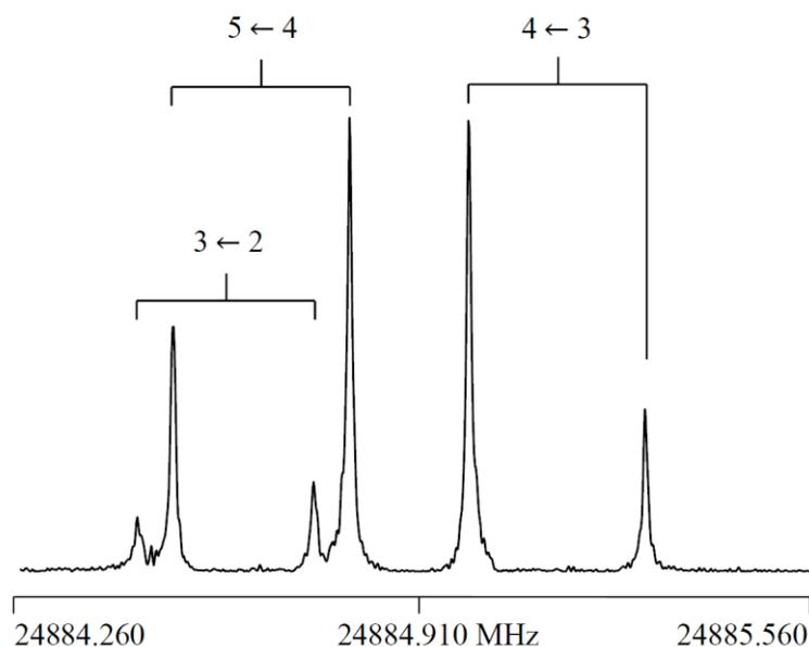
**Figure 2.** A high resolution spectrum of the  $4_{14} \leftarrow 3_{03}$  A species transition of 2MP. The Doppler doublets are marked by brackets. The quantum numbers  $F' \leftarrow F$  are given at the respective
