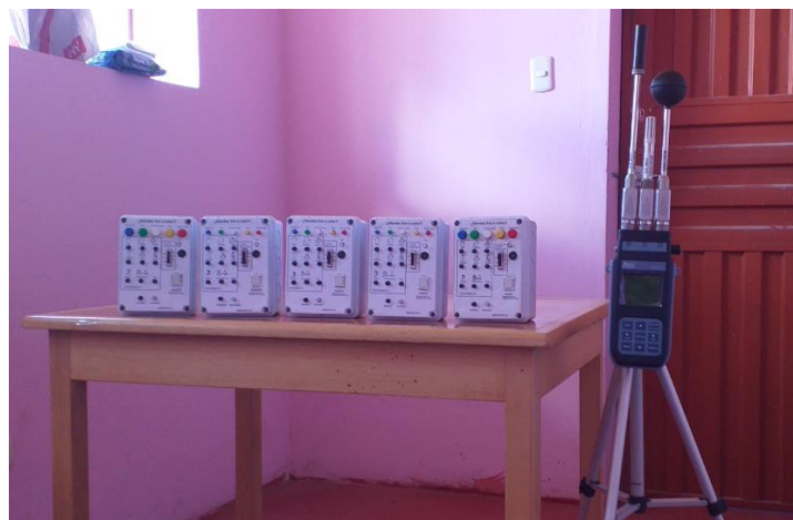
Figure 5. Photographs of DeltaOhm HD 32.3 and implemented devices in an indoor environment at the time of calibration in the village of Imata.
