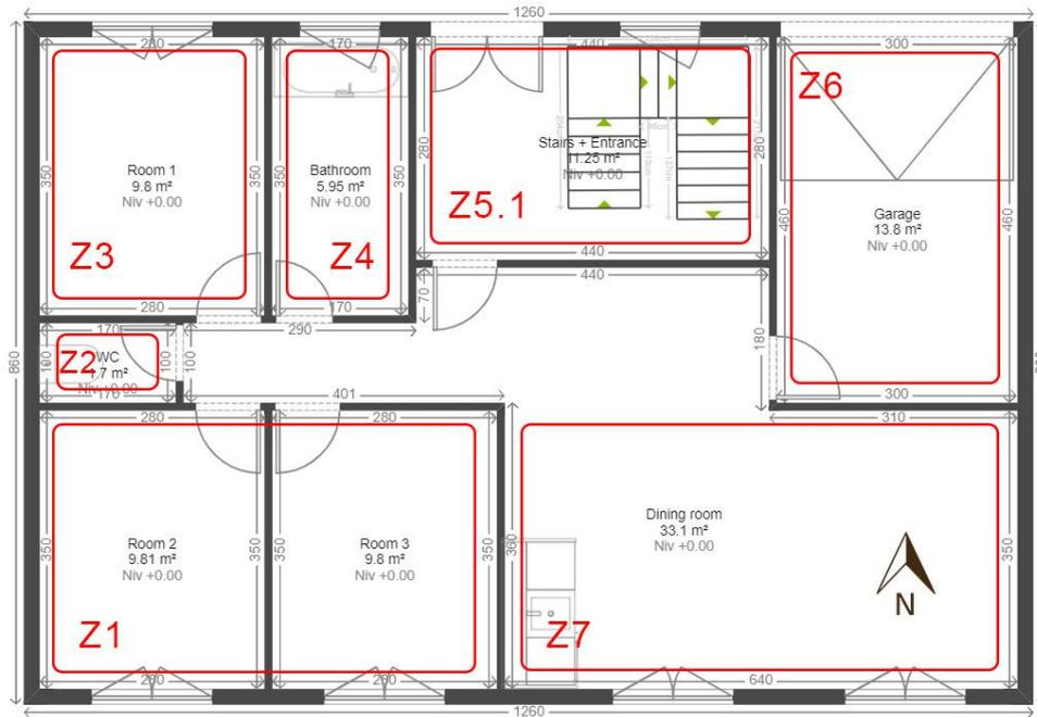
**Fig. 3. Ground floor 2D plan and thermal zoning.**
