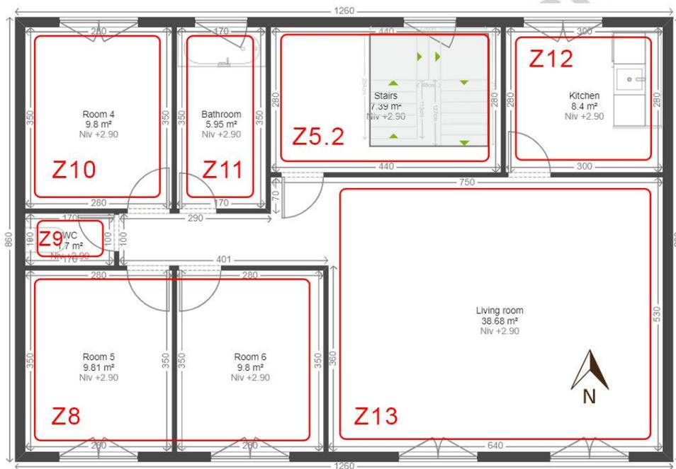
**Fig. 4. 1st floor 2D plan and thermal zoning.**
