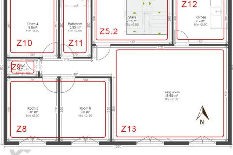
Fig. 4. 1st floor 2D plan and thermal zoning.
