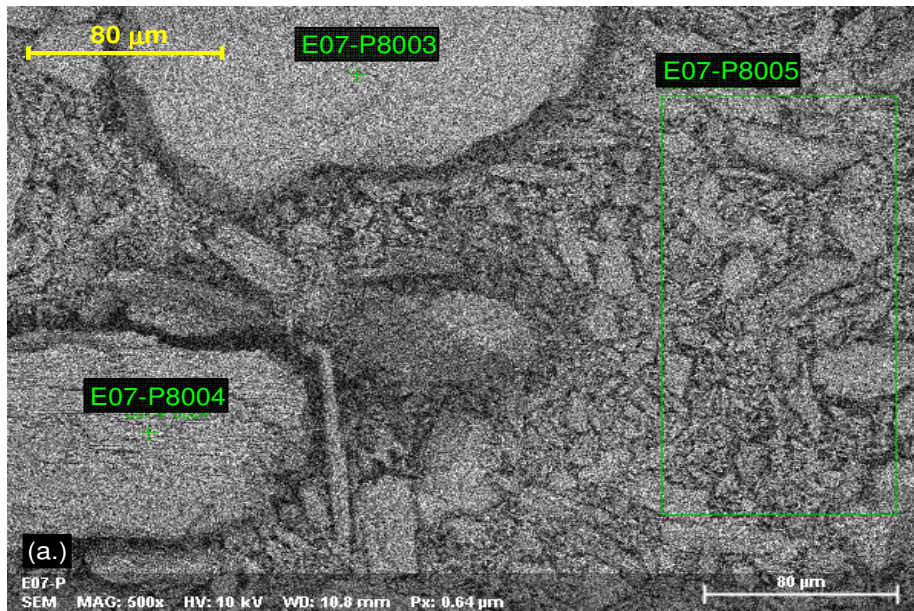
4 5 6 Fig. 3 SEM micrograph of used plaster
