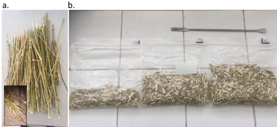
Fig. 2 Moroccan hemp: (a) stalks (b) fibers used during the sample preparation
