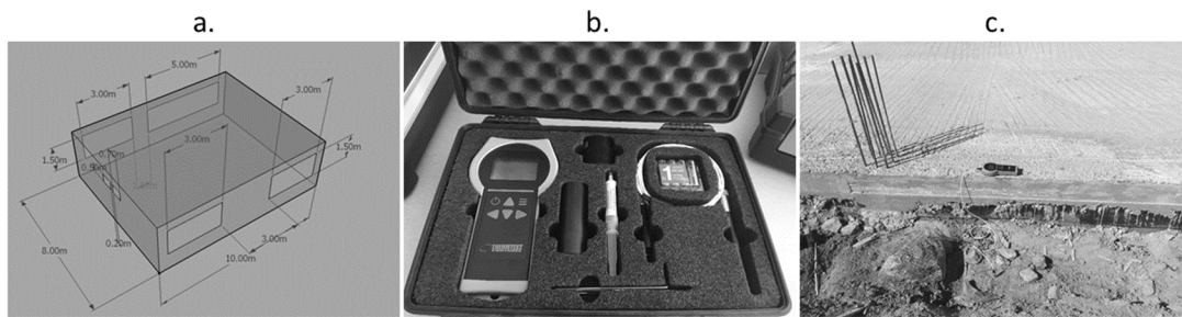
8 9 Fig. 16 Studied building: (a) 3D sketch plan (b) TLS-100 soil conductivity meter (c) Measuring place.
