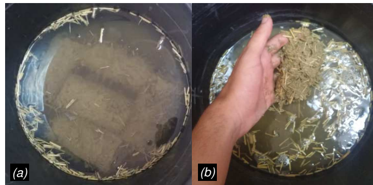
6 7 Fig. 18. Water absorption test by total immersion of PS-adobes (Top View).
