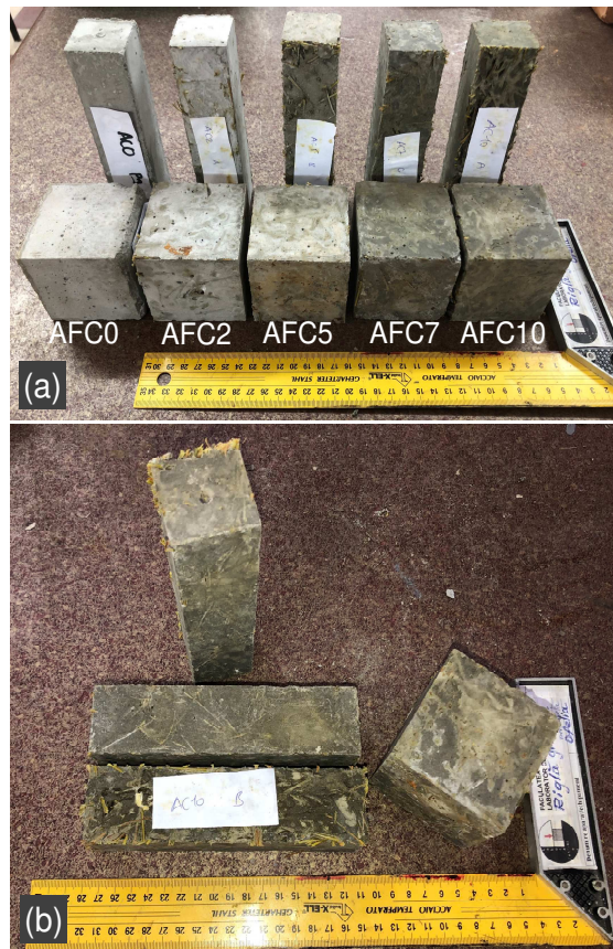
Fig. 5. Photographs of prepared specimens (a) AFC mixes (b) AFC10.
