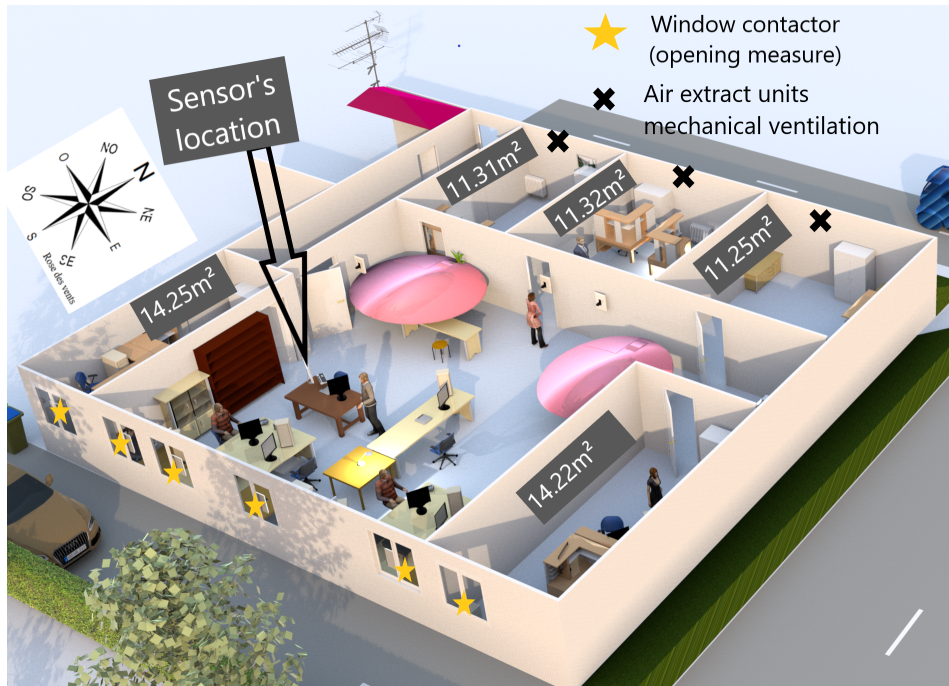
Figure 1: Plan of the office space ( 132 \text{ m}^2 , 364 \text{ m}^3 ). The configuration of the tables varies with the number of occupants. An example of motion detection is materialized by two pink half spheres.
