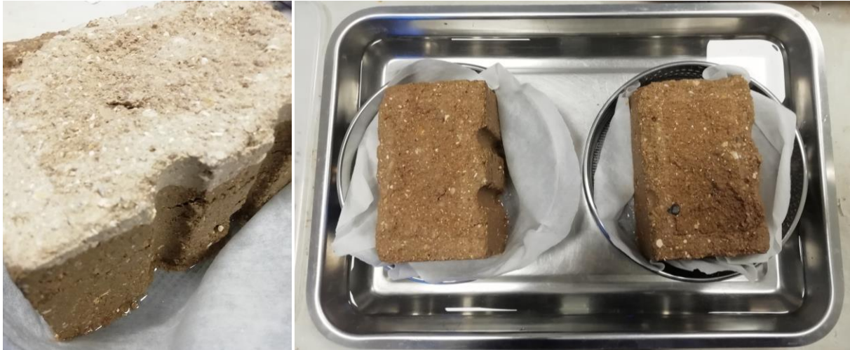
Figure 3. Capillary water absorption test for CEB samples
